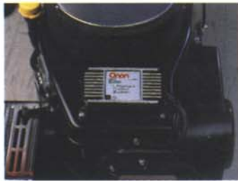
The Onan Emissions Control System featured on the 14 hp model.
